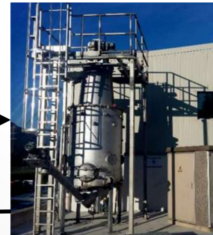
Entrained flow carburettor Wood / Coal Gasifier
