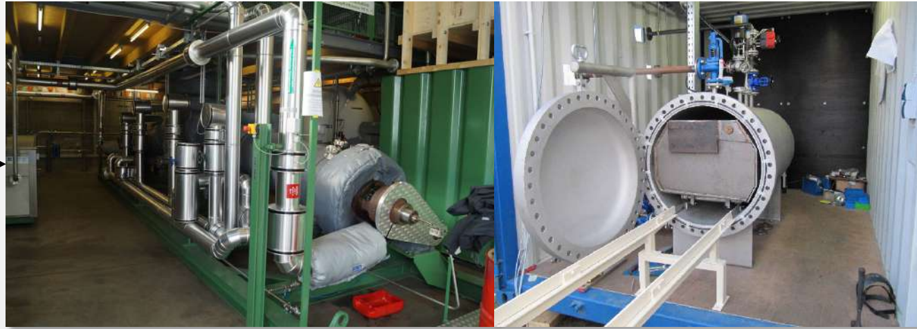
HTC-Reactor (< 30% DM) or VTC-Reactor (> 30% DM)
